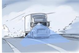
Automation of individual function, driver fully engaged – Driver may be "feet off" (when using ACC) or "hands off" (when using Lane Keep Assist)
