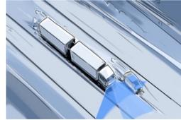
Automation of multiple functions, driver fully engaged – Driver may be both "feet-off" and "hands off", but eyes must stay on the road
