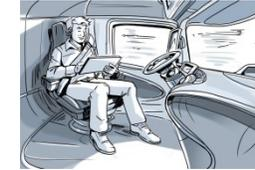
Automated in certain conditions, driver not expected to monitor road – Vehicle can operate without a driver in specific situations, e.g. highway driving
